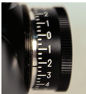
Figure 8. Click calibrated Windage Knob (0-10-0)
