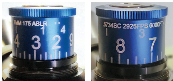
Figure 17. Dialing the BDC Turret from 200 to 725 yards
