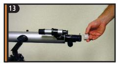
Loosen the set screw on the focuser so that it does not obstruct the inner diameter of the focuser. Remove the plastic cap covering the end of the focuser.
