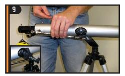
Insert the slow motion control rod into the hole on the mount.
