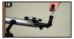
Insert the chrome barrel of the 20mm eyepiece into the barlow and tighten the set screw to secure in place.
