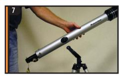
Locate the optical tube and line up the tube with the holes on the mount.
