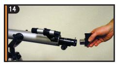
Locate the diagonal and remove the plastic covers. Insert the chrome barrel of the diagonal into the focuser and secure in place by tightening the set screw.
