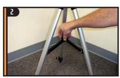
To set up the tripod, spread the legs outward until they are fully extended and push down center locking brace. Extend the center portion of each of the three tripod legs down 6-8".
